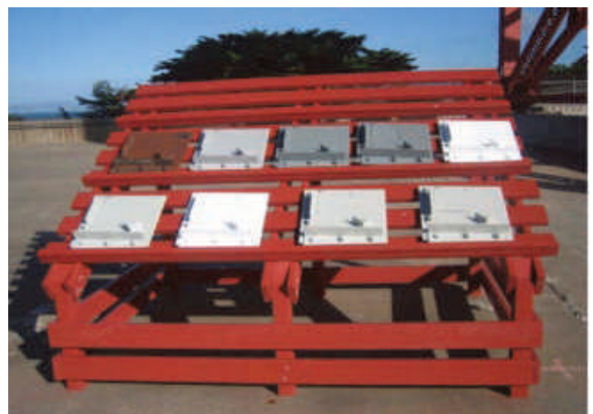
Fig. 3: Type II panels deployed at the Golden Gate Bridge
